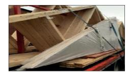
8. The driver can assist the responsible person to cut the 8mm blue rope attaching the panel to the vehicle centre bars if required. This must be carried out from a safe position using a telescopic cutting device.
